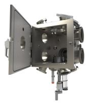
The QBox 400 is a high vacuum, front loading box style deposition chamber that is engineered for easy access to all components of the system to provide rapid maintenance and loading cycles. The chamber is outfitted will all conflat flanges for easy instrument integration. All deposition source ports are in a confocal arrangement to optimize deposition uniformity and coverage.
